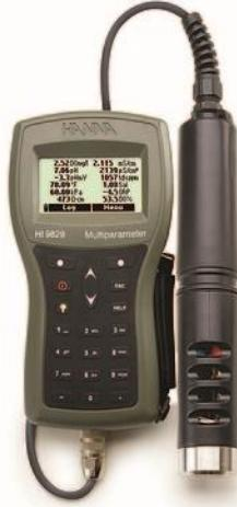
A photograph of a handheld multiparameter device. It has a digital display showing various measurement values and a keypad with buttons for navigating menus. A probe is connected to the side of the unit, which is used for immersing it into liquids to take readings. |
