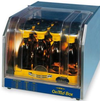
A photograph of an Oxitop Box, a blue rectangular apparatus designed for simultaneous BOD analysis. It contains several brown glass bottles arranged in a tray, with a clear cover on top. The brand name 'OXITOP' and 'Box' is visible on the front panel. |
